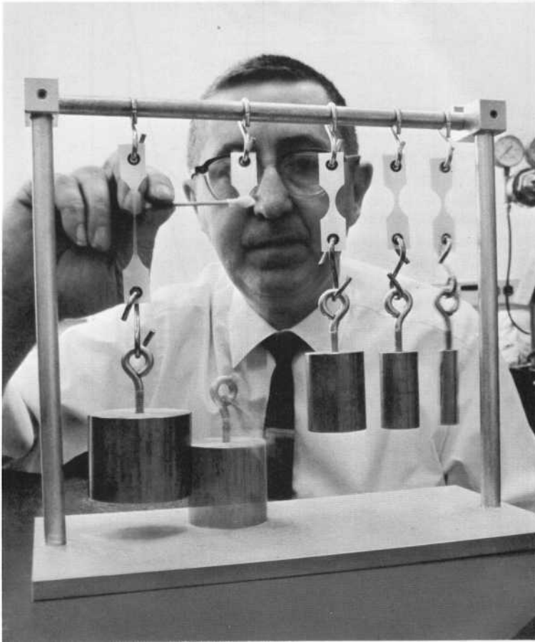
The first three polyethylene strips, right to left, are stressed below their yield points, the fourth is at the yield point, and the elongated one is stressed much beyond its yield point. As H. M. Gilroy, Member of Technical Staff, applies an active agent to each of the strips, only the one stressed at its yield point breaks.
